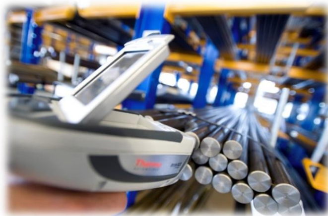
Identification test of raw material by X-ray fluorescence analysis (XRF)
